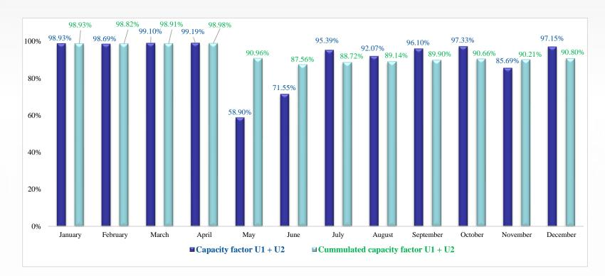
\*Unit 2 entered the planned outage program on 07 May 2023, in order to carry out the planned maintenance works, the synchronization to the National Power System (NPS) being realized on 15 June 2023.
